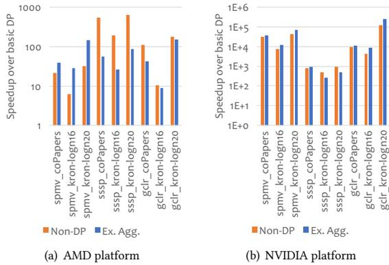
**Figure 4: Speedup of the implementations without dynamic parallelism (Non-DP) and the implementations with existing subtask aggregation (Ex. Agg.) over the default dynamic parallelism implementations (Basic DP).**
