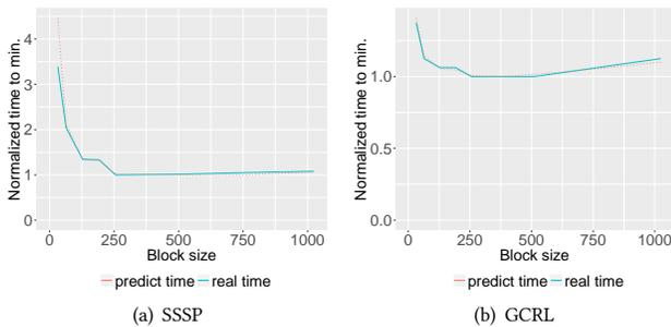
**Figure 13: The result of the performance prediction of SSSP and GCLR algorithms *kron-logn16* dataset, task size = 128 and number of tasks = 64 (normalized to minimal time)**
