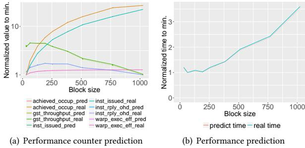
**Figure 12: The result of the performance prediction of the SpMV algorithm with *kron-logn16* dataset, task size = 128 and number of tasks = 64 (normalized to minimal time)**
