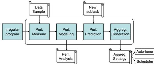
**Figure 8: Architecture of our adaptive subtask aggregation**
