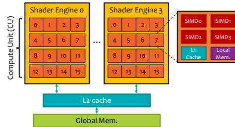
Figure 1: AMD GPU Architecture Codenamed “Vega”
