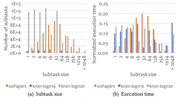
**Figure 6: The distribution of subtask size and execution time of the SpMV algorithm. The execution time of each subtask size is normalized to the total execution time.**
