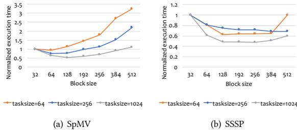
**Figure 7: Performance of SpMV and SSSP algorithms with different block size. The execution time is normalized to that of block size = 32.**
