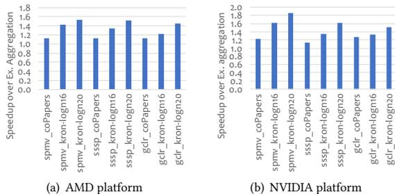
**Figure 14: Speedup of the optimal subtask aggregation over the existing subtask aggregation (Ex. Agg.)**
