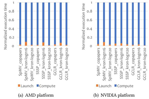
**Figure 5: Breakdown of the child kernel execution time in the existing subtask aggregation mechanism (Ex. Agg.).**
