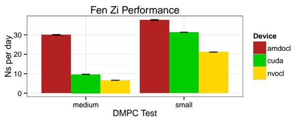
**Figure 5: A comparison of nanoseconds of simulation time performed per day (reported by Fen Zi).**
