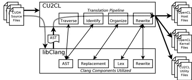
**Figure 1: Architecture of CU2CL and its relationship to Clang.**
