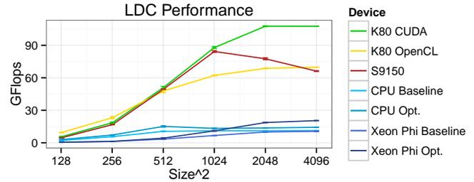
Figure 3: Reported GFlops achieved within the iterative loop of the LDC simulation as a function of problem size and compute device.
