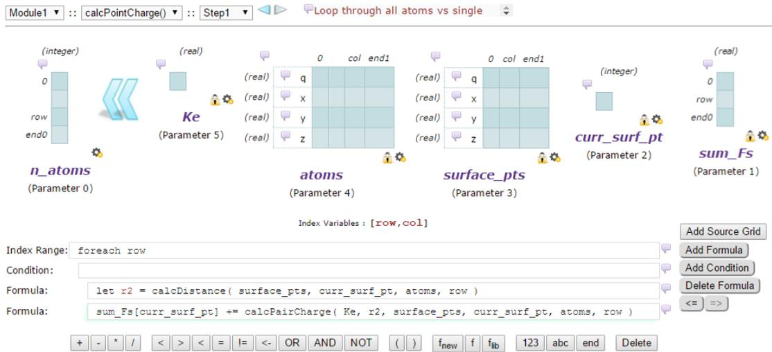
Figure 2: GLAF graphical programming interface (GPI) [15]
