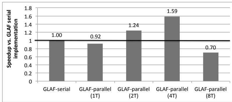
**Figure 6: Parallel scalability: Speed-up of fastest GLAF-generated version (*GLAF-parallel v3*) with varying number of threads (*T*) versus GLAF serial implementation of Synoptic SARB kernels of interest**
