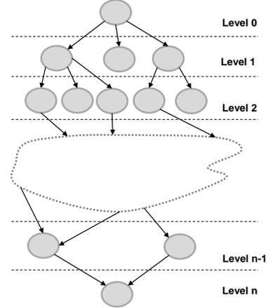
Fig. 4: The application ASAP schedule on a theoretical architecture with infinite resources
