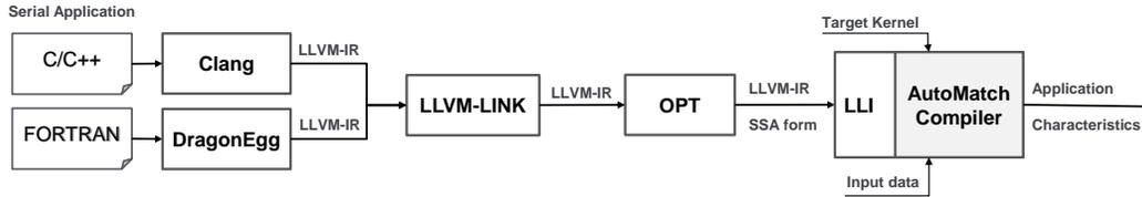
Fig. 3: The design and implementation of AutoMatch compiler
