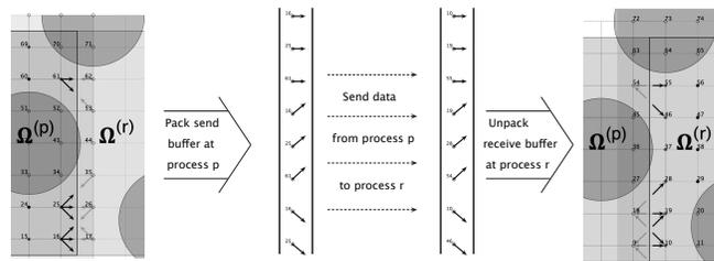
Figure 4. Graphical depiction of the MPI communication pattern along a boundary for the LBM. Communicated distributions are packed into contiguous send buffers on the GPU, ignoring lattice sites at any  $\mathbf{x}_i \in \Omega_s$ . The data is then sent to the neighboring process and unpacked to the appropriate location on the GPU.
