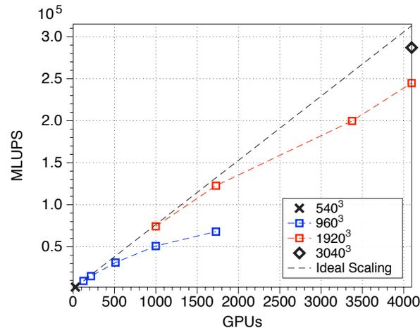
Figure 6. Scaling results obtained for several domain sizes on Titan, including strong scaling for both a  $960^3$  lattice and a  $1920^3$  lattice. Ideal scaling is shown based on a  $540^3$  simulation performed on 27 GPU. Results are reported in million-lattice-node updates per second (MLUPS).
