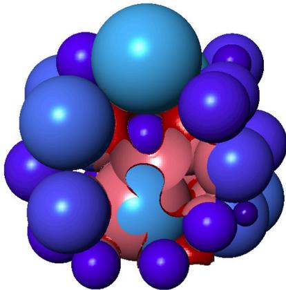
Figure 5. Closeup view of a multiphase interfacial configuration in a sub-region of a sphere packing. The  $wn$  interface  $\Omega_{wn}$  (red) and the  $ns$  interface  $\Omega_{ns}$  (pink) are also shown, constructed using the PMMC algorithm. The solid spheres are also depicted.
