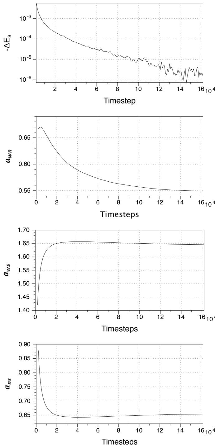
Figure 7. Interfacial area and surface energy measurements conducted during a multiphase flow simulation within a packing 11,402 spheres on a lattice size of  $1200^3$ . Area measurements were calculated every  $10^3$  time steps and the duration of the simulation was 163,000 time steps.
