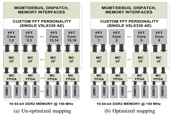
Figure 2: FFT mapping on the Convey HC-1
