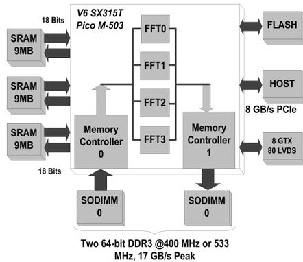
Figure 3: FFT mapping on the Pico M-503
