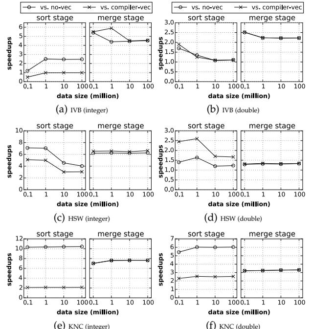
Fig. 12: ASPaS vs. *icpc* optimized (“compiler-vec”) and serial (“no-vec”) codes. For the *merge* stages, the lines of “compiler-vec” and “no-vec” usually overlap.
