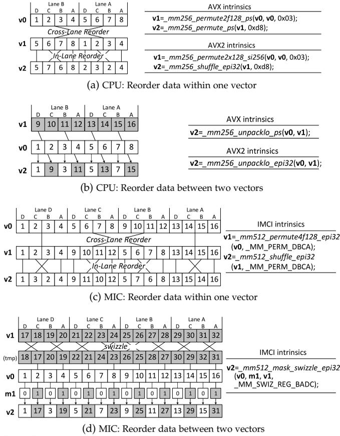
Fig. 1: Rearrange data on Intel CPU and MIC from: (a,c) the same vector register with the permute and shuffle instructions; (b,d) two vector registers with the specific unpack instructions on CPU or masked swizzle instructions on MIC
