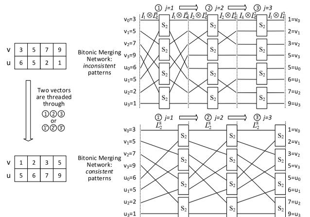
Fig. 7: Two formalized variants of bitonic merging networks: the inconsistent pattern and the consistent pattern. All elements in vector  $v$  and  $u$  are sorted, but inverted in vector  $u$ .
