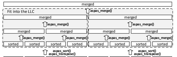
Fig. 10: The organization of ASPaS kernels for the **single-threaded** `aspas::sort`
