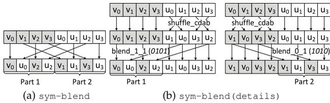
Fig. 9: Symmetric blend operation and its pairing details
