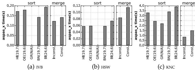
Fig. 11: Performance comparison of *aspas\_sort* and *aspas\_merge* with different sorting and merging networks. The kernels are repeated by 10 million times over a built-in vector-length array and total times are reported. The numbers of comparators and groups are given in parenthesis for sorting networks.
