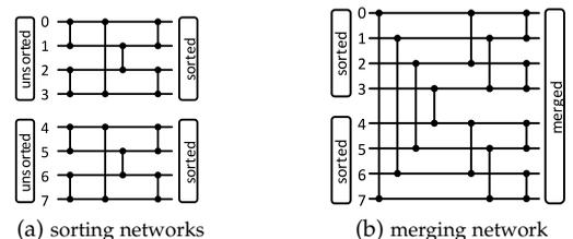
Fig. 2: Bitonic sorting and merging networks (a) Two 4-key sorting networks (b) One 8-key merging network
