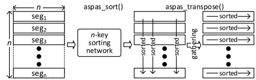
Fig. 4: Mechanism of the sort stage: operations generated by *SIMD Sorter* and *SIMD Transposer*
