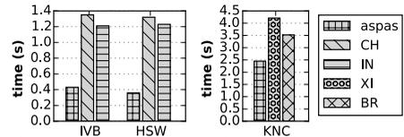
Fig. 13: ASPaS kernels vs. Previous manual approaches. We repeatedly (1 million times) sort  $8 \times 8 = 64$  integers for CPUs and  $16 \times 16 = 256$  integers for MICs, respectively. The time on data load from memory to registers and store from registers to memory are included with the sort and merge in registers.
