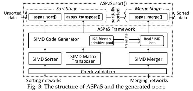
Fig. 3: The structure of ASPaS and the generated sort
