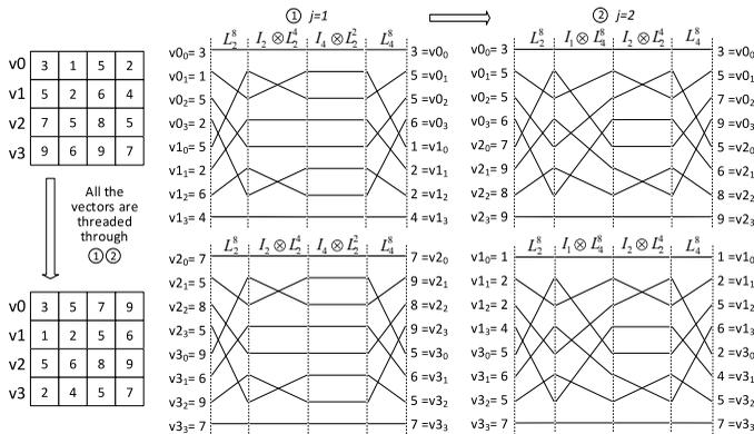
Fig. 6: Four 4-element vectors transpose with the formalized permutation operators of DSL.
